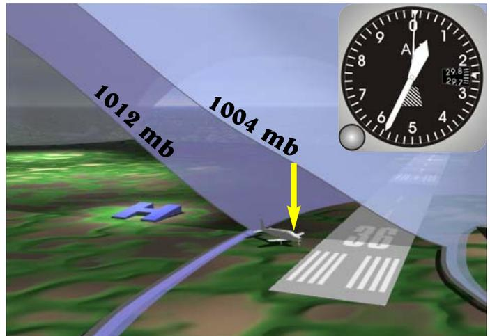
Figure 9b During the day the high pressure draws closer, and the 1012 mb (29.88 in. Hg) pressure surface arrives. The altimeter now reads 230 ft MSL lower. The 1004 mb pressure surface is above the airport. So the altimeter is below that surface and indicates a lower altitude relative to that 1004 mb surface..
