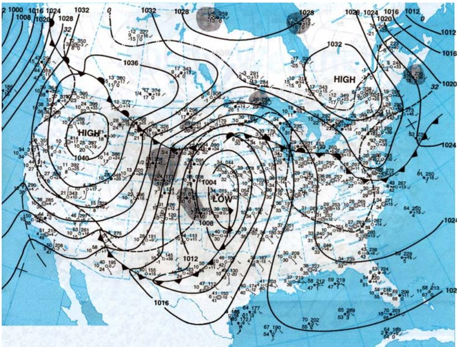
Figure 4. Areas of high and low pressure result from the atmosphere's attempt to redistribute excesses and deficiencies of heat and mass. Strong storms develop and promote rising air. Next to these storms, areas of high pressure with descending or subsiding air complete the process. Depicted here are conditions for 1200 UTC on February 9, 2002. The lines are isobars or lines of equal sea level pressure. The units are millibars, an international unit for pressure measurement.
