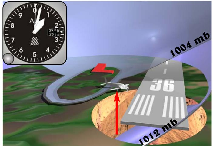
Figure 8b During the day, the low pressure center arrives with the 1004 mb (29.65 in Hg) pressure surface. At the end of a long day and without changing the setting in the Kollsman window, the altimeter now reads 230 ft MSL higher. The pressure has fallen 8 mb (0.23 in Hg). The altimeter reads 230 feet higher because the 1012 mb pressure surface is “below” the field.
