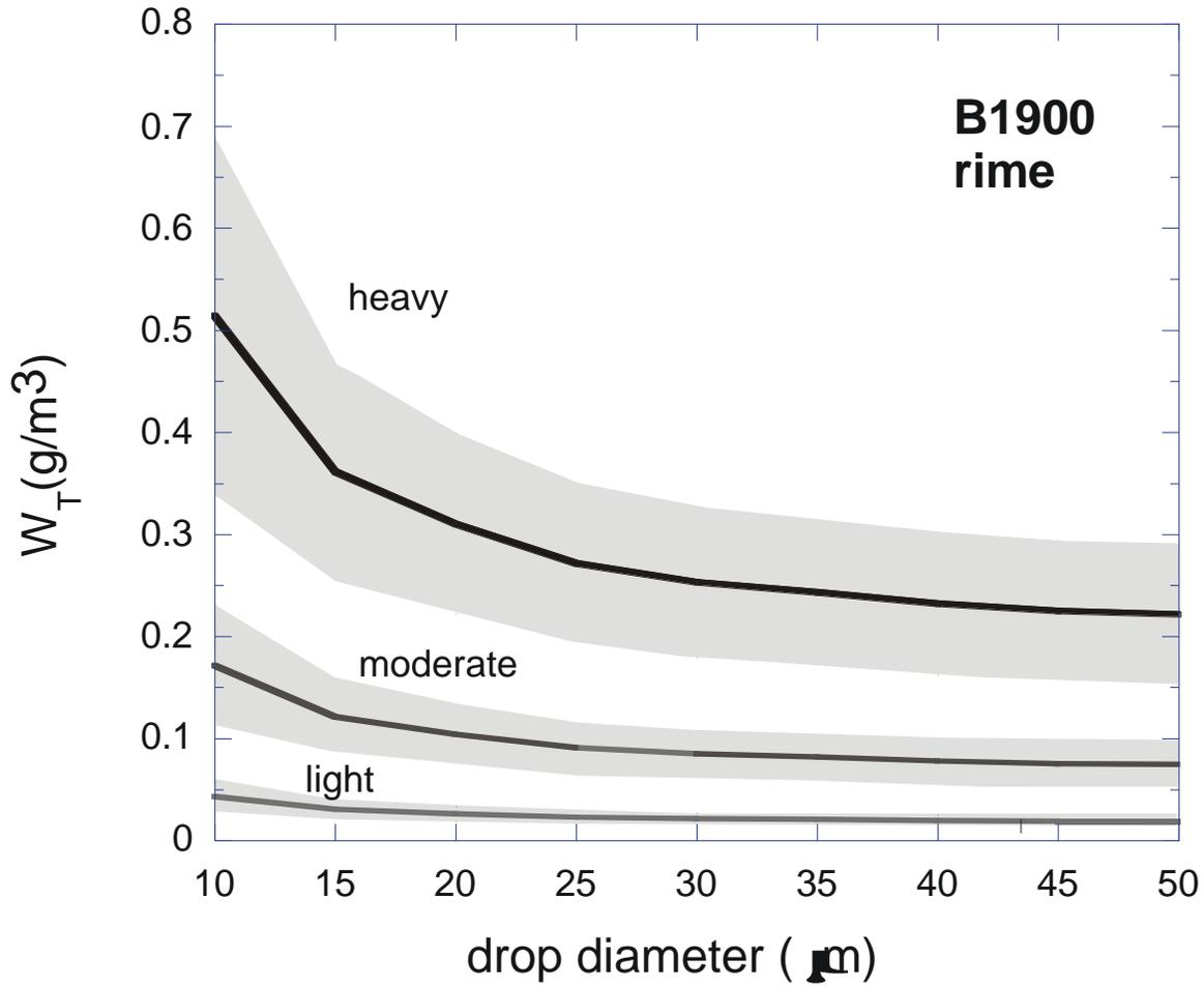
Figure 1: Dependence of threshold liquid water contents on drop diameter for rime ice on the B1900. The median volume diameter is assumed 15  $\mu\text{m}$ . The shaded areas represent uncertainty envelopes as listed in Table 2.
