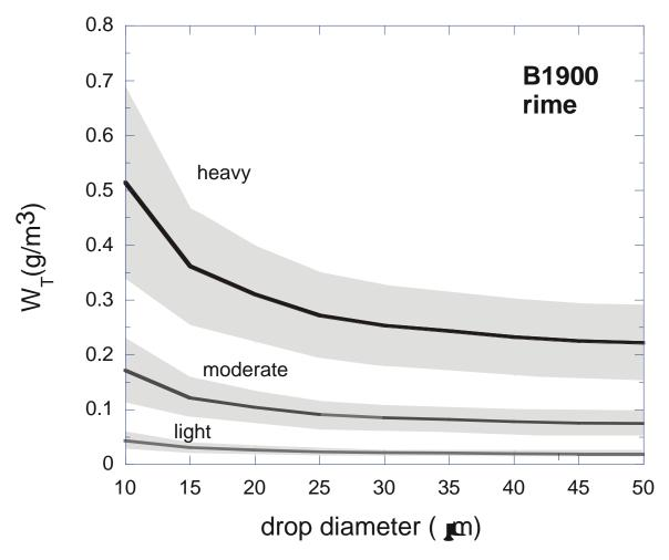
Figure 1: Dependence of threshold liquid water contents on drop diameter for rime ice on the B1900. The median volume diameter is assumed 15  $\mu$ m. The shaded areas represent uncertainty envelopes as listed in Table 2.
