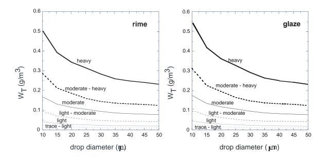
Figure 3: Expected icing intensity expressed as liquid water content threshold  $W_T$  versus drop diameter for rime and glaze icing of all collectors listed in Table 2.
